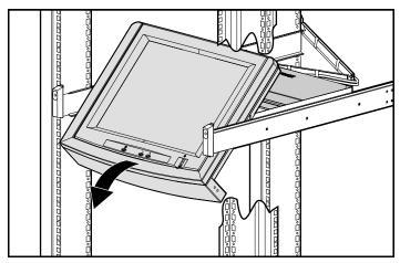
Figure 2-13. Setting the monitor viewing angle
